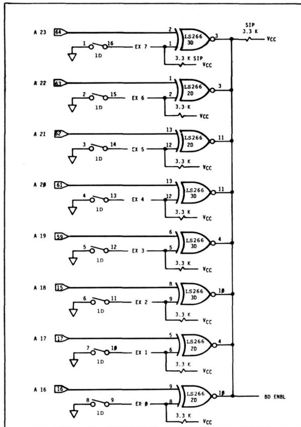
When the switches are set to the appropriate Address, that Address and the Address generated by the CPU must be identical for the board to be enabled. If the switch is set to the ON position the CPU generated address must be low, likewise if the switch is set to the OFF position the CPU address must be be a high level. As in the block enables, ALL addresses must match the switch settings before the board will recognize an address generated by the CPU.
